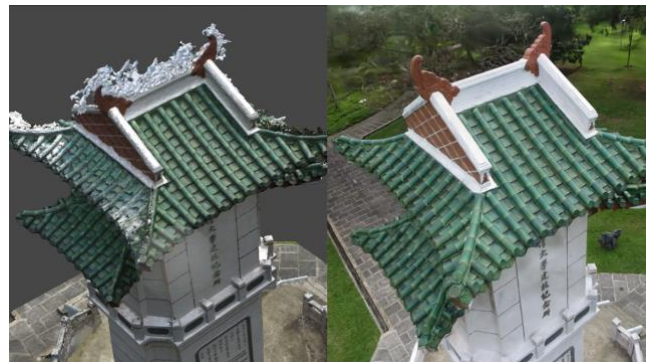
Figure 6. Comparison of photogrammetry (left) and Gaussian Splatting (right) from identical dataset. ©The authors.
