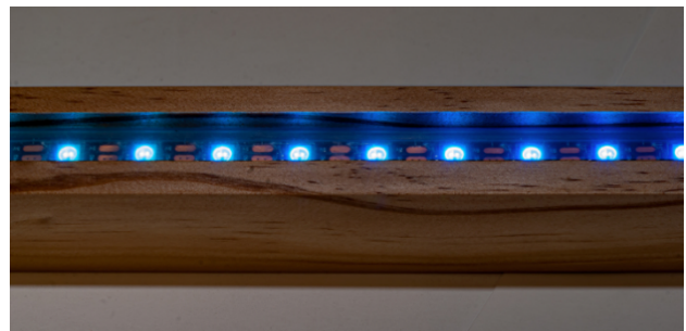
Figure 2. A section of LEDs inlaid on a Thing-onna-Stick. © 2015 Author.
