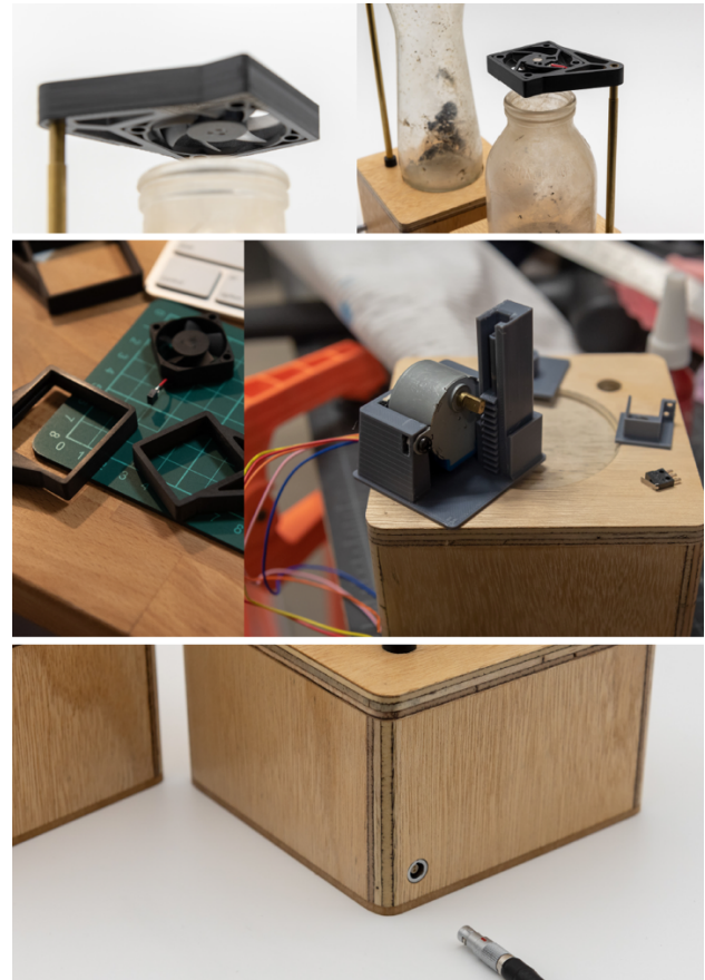
Figure 4. Various technological components augmented the found glass bottles, from top to bottom: electric fans on the reciprocating stems; 3D printed fan housing and stepper motor holders; the use of wood to complement the glass bottle and brass stem, and the appliance-like power connector to convey ease of use. © 2018 Author.
