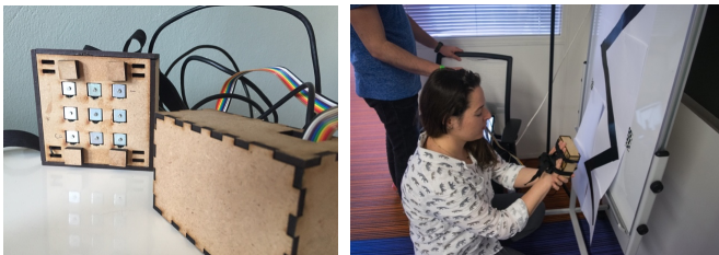
Figure 2: A low-resolution portable interface with 9 motorized pixels using solenoids and a camera input. This interface was flexible in placement.
