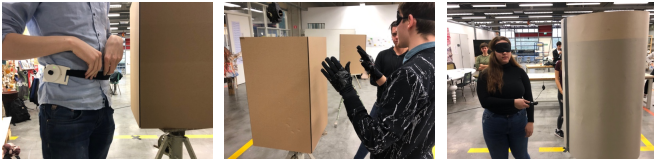
Figure 4: Three different interfaces were used in a blindfolded experiment to recognize 3-dimensional cardboard shapes. All three devices translated distance into vibration intensity. Left: Hip-worn double device. Middle: Hand-held double device. Right: Hand-held single device.
