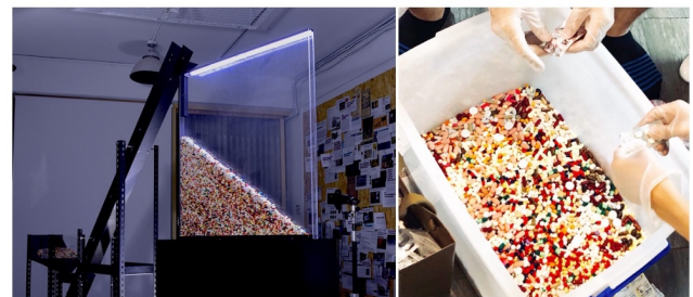
Figure 3. Left: The mechanical system used in transporting particles to the top of the container initiating avalanche events. Right: The recycled pills are collected and unpackaged.
