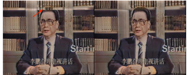
Fig 2. Result of clearing Large Area Defects known as Head Clogging
