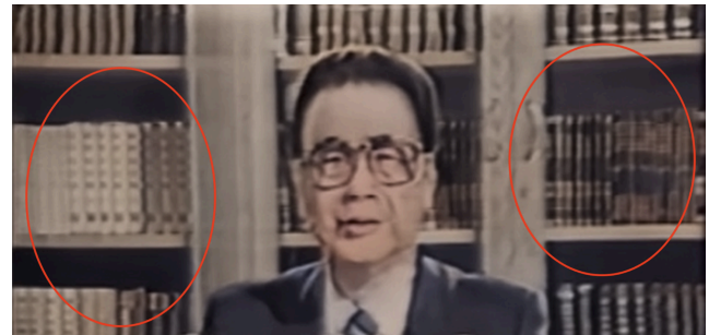
Fig 5. Upscaling result (480i to 4K UHD) using Lanczos kernel.
