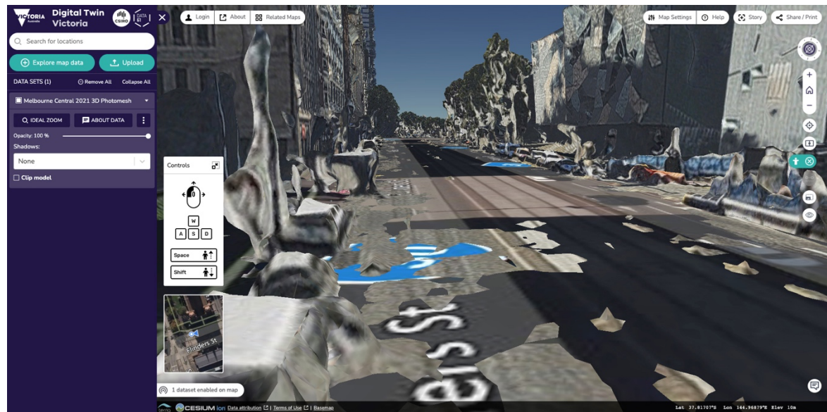
Figure 6: Digital Twin Victoria screenshot, Melbourne Central 2021 3D Photomesh, shows a blobby, fractured view of the street in Pedestrian mode. Screenshot taken by the author.
