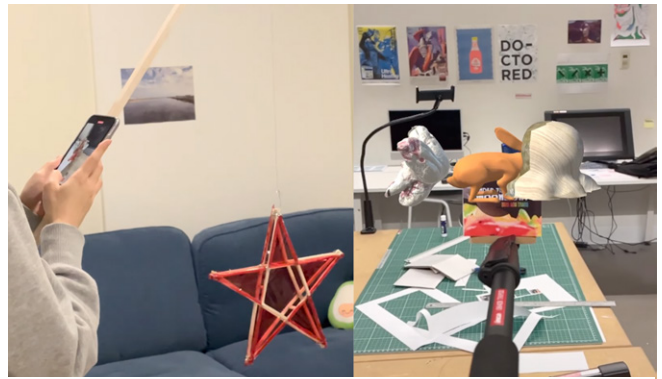
Figure 7. Phone attached to lantern stick (left), and tracking of fiducial marker for lantern recognition (right)
