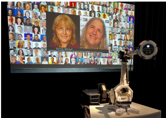
Figure 4. Yamin Xu’s AI Connections Robot tracks human faces and matches them with photos from the archive.
