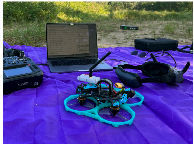
Figure 5. Transmitter piggyback configuration and other components of the system at Nam Sang Wai. ©Samuel Swope. 2023
