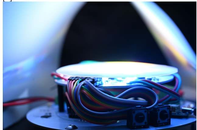
Figure 4 Multi-spectral LED module to reproduce spectral light data as a performance tool with view of testing apparatus
