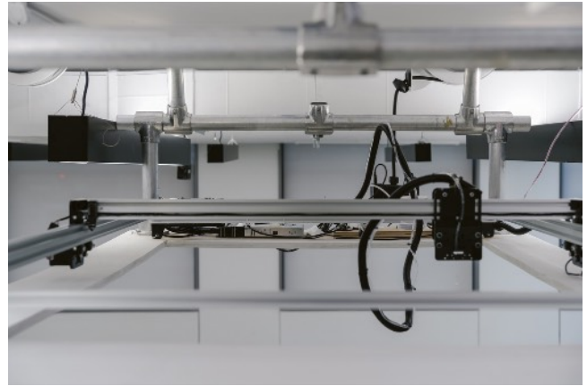
Figure 8. CNC Water Dripping Mechanism © Yan Shao
