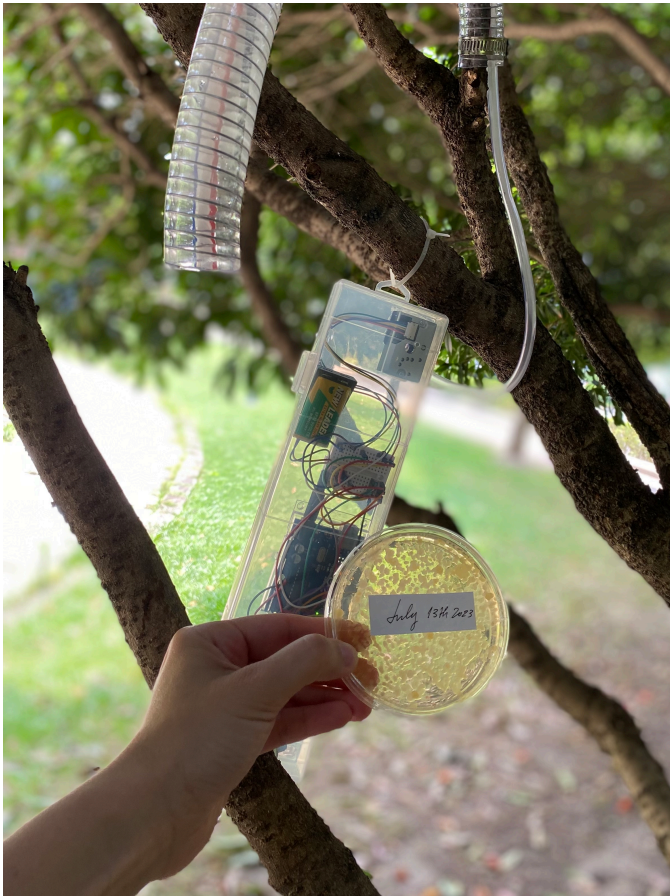
Figure 3. “Inhaling Consciousness: Talking Through Tubes” (2023-2024) — tube (tree’s branch prosthesis to blow the breath through) and secondary tube that enters the detection area of the GP2Y1010AU0F sensor that sends input (data) to the Arduino and attached LCD for ‘performative data-visualization’. Image by the author.
