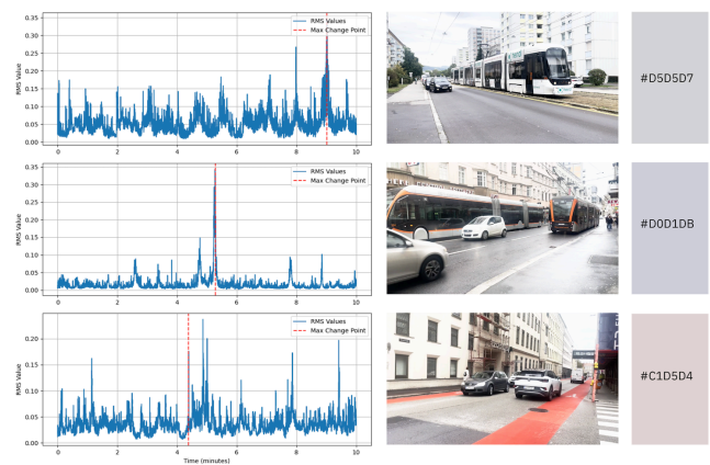
Figure 3. Composite analysis of audio-visual data extracted from a 10-minute HD video. The left column displays line plots of RMS audio values, with a red line marking the point of maximal change within a 30-frame window. The central column captures the corresponding video frames at these points, while the right column features the color patches with their respective hexadecimal codes, representing the mean-averaged color value from each identified video frame.
