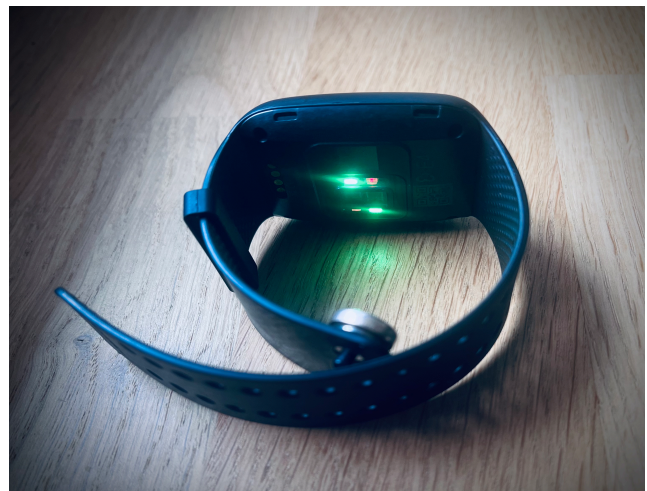
Figure 1. Empatica E4 equipped with 4 sensors (EDA, BVP, thermometer and accelerometer). The green and red light emitted is from the BVP sensor that measures the amount of blood present in the tissue.
