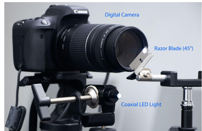
Figure 4. Camera lens, razor, and LED light position settings, for a schlieren setup to visualize refractive index changes of transpiration vapor coming out from plant leaf-tips
