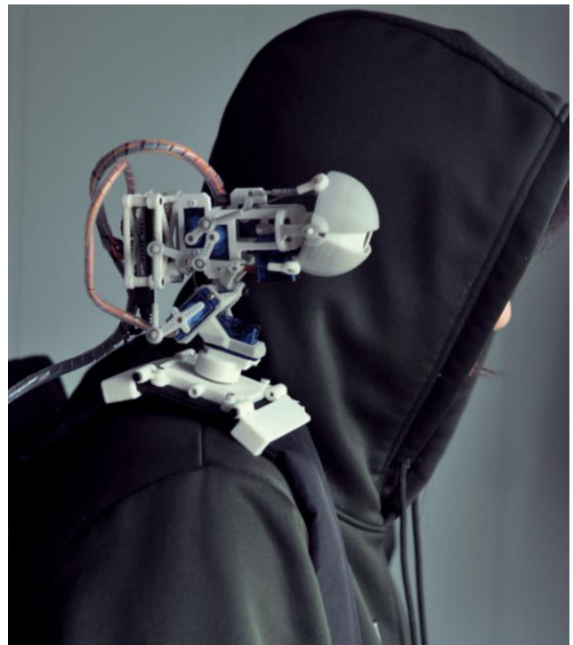
Figure 1. Iris, a wearable robot has a heart rate sensor connect to the wearer to share feelings with the wearer.
