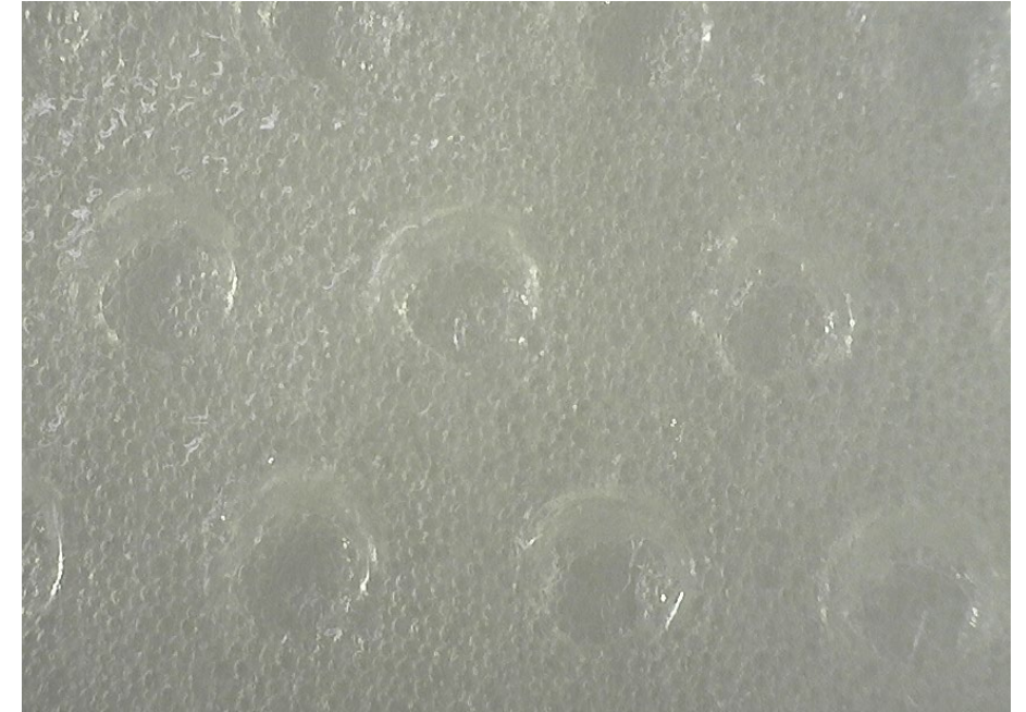
Higher magnified image of perforated silicone interface layer on top of absorbent layer
