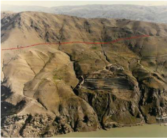
Figure 30. Overview of Cairnmuir Slide. The red line is the inferred geological terrane boundary fault (Contact Energy Ltd).
