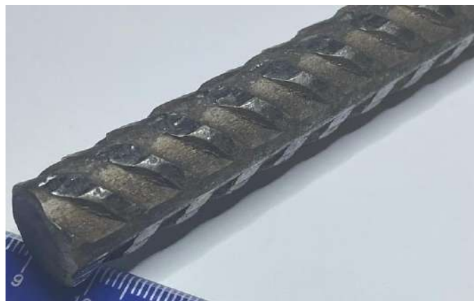
Figure 3 Damage to Rib profile due to decoiling
