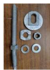
Figure 18. Typical bolt shear and toothed washer splitting failure mode C2 test M20 Anchor Stud 16mm Plt – Orientation 1
