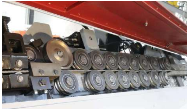
(b) Typical bar straightening process
