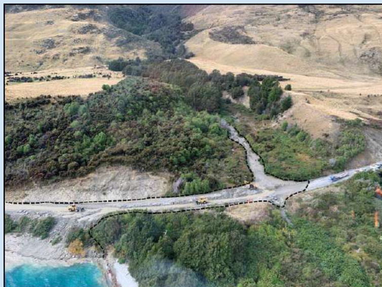
Figure 3: Left: May 2010 rockfall at the Narrows (photo: ODT). Right: Aerial view of debris flow impacts at the Queenstown-Glenorchy road, annotated to show the approximate extent of debris deposition (photo provided by Maddi Phillips, WSP Ltd).
