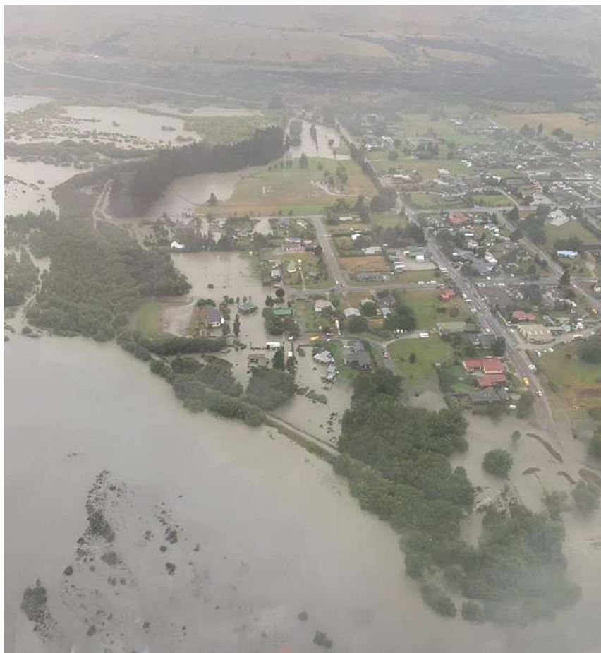
Figure 6: Flooding of Glenorchy township residential area, due to high Rees River flows causing overtopping of a section of the Rees-Glenorchy floodbank (February 2020).
