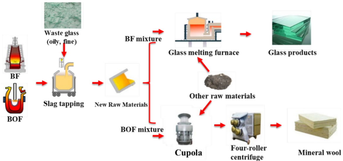
FIG 7- Conversion of wastes to new raw materials for glass and mineral-wool manufacturing
