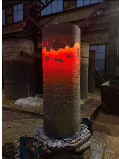
FIG 3 – The ESR ingot remelted by model slag
