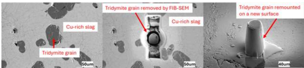
FIG 3 Demonstration of removing and remounting of targeted phase for EPMA analysis to eliminate the SBF effect.
