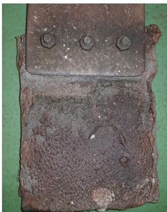
FIG 2 – Appearance of the cathode sample after electrolysis.
