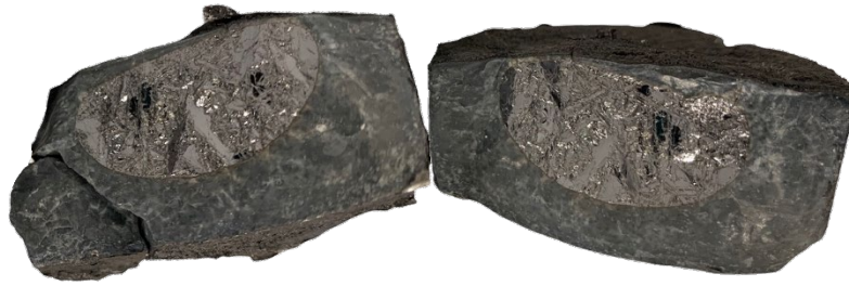
FIG 6 - Physical structure of the product obtained from the experiment using \text{CaF}_2 in prefused slag and pure aluminium as a reductant.
