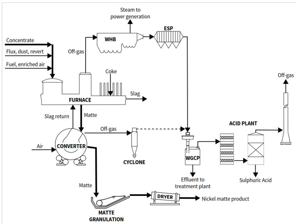
FIG 1 – Process Flow Diagram of Kalgoorlie Nickel Smelter
