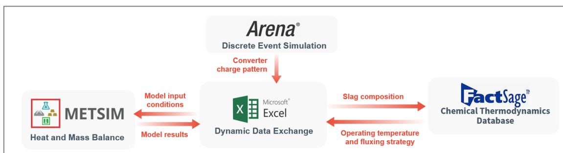
FIG 4 – Modelling Software Integration Diagram
