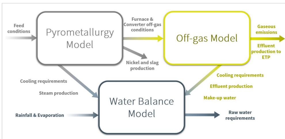
FIG 3 – Interconnection between METSIM models
