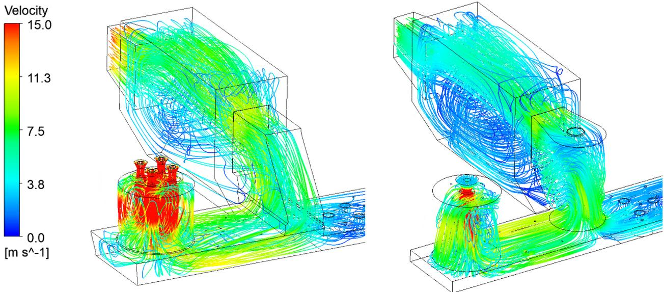
FIG 5 – CFD Velocity Comparison (Left: Existing, Right: Upgrade Option)
