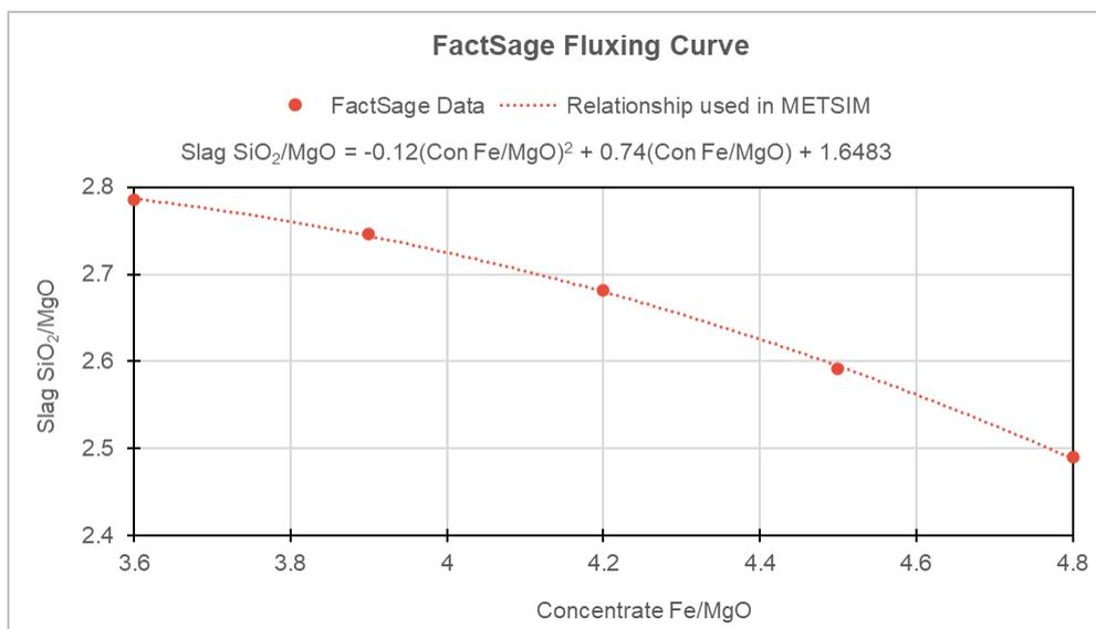
FIG 2 – Example fluxing curve generated using FactSage
