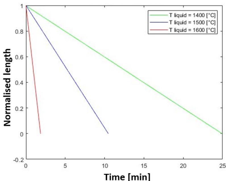
FIG 4 – The influence of hot metal temperature on melting behaviour of small scrap (From right to left 1400°C, 1500°C and 1600°C).
