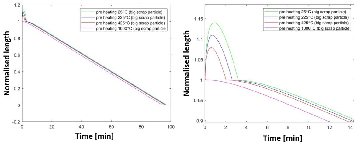
FIG 6 – (a) The influence of pre-heating temperature on melting behaviour of large scrap (b) Magnification of the early stage of the melting
