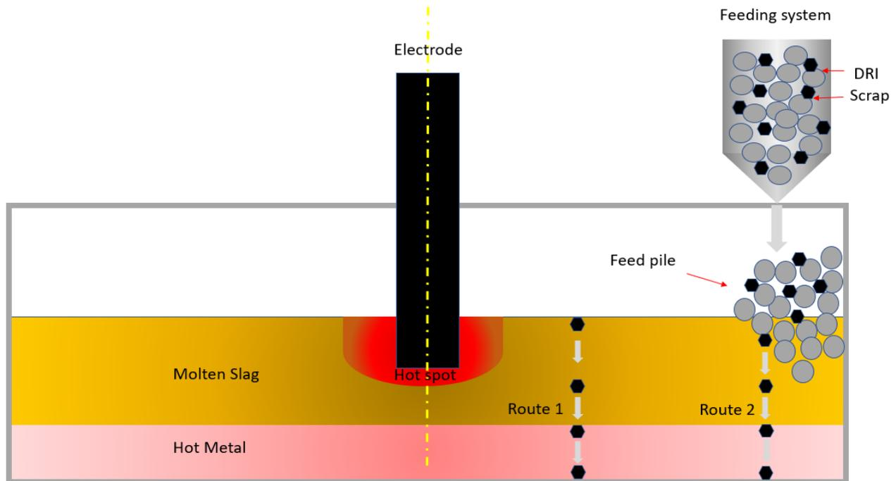
FIG 1. Schematic of an OSBF cross section. Left circles represents direct charging through slag; right circles show charging through feed pile.
