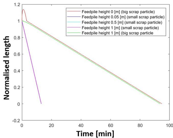
FIG 5 – The influence of scrap size for different feed pile height on melting behaviour of scrap
