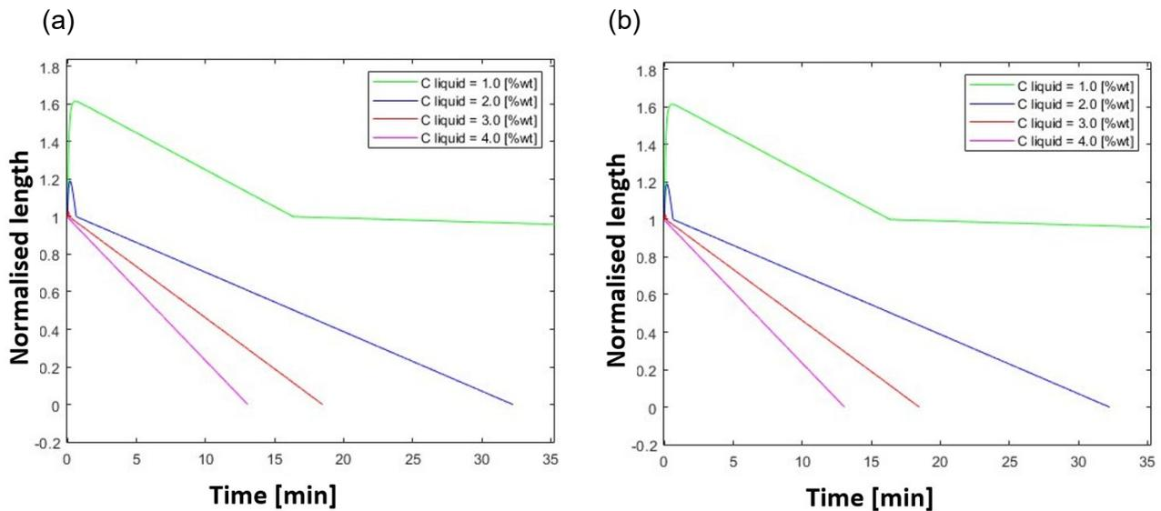
FIG 3 – (a) The influence of carbon concentration in hot metal on melting behaviour of small scrap particle (b) Magnification of the early stage of the melting
