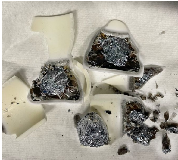
FIG 7 - Silicon-slag sample after 1 st stage of slag treatment at 1550 °C for 2 hours. A big portion of the silicon was taken for 2 nd stage of slag treatment.
