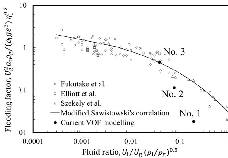
FIG 13 – Flooding data of published works (Dong *et al*, 2009), calculated ( $FR$ ,  $FF$ ) points for cases with different gas inlet velocities.
