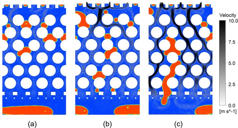
FIG 12 — Simulated counter-current gas and slag flow in the packed bed at time  $t = 9.5$  s for different superficial gas velocities: (a) 0.33  $\text{m}\cdot\text{s}^{-1}$ , (b) 0.82  $\text{m}\cdot\text{s}^{-1}$ , and (c) 1.64  $\text{m}\cdot\text{s}^{-1}$ . Note that the legend is used for gas velocity.
