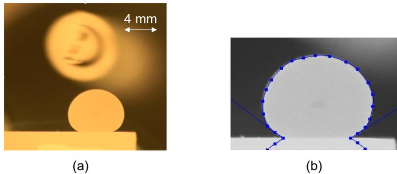
FIG 5 – Depiction of contact angle measurement: (a) original image captured from video, and (b) drop analysis using Image J software with DropSnake plugin.
