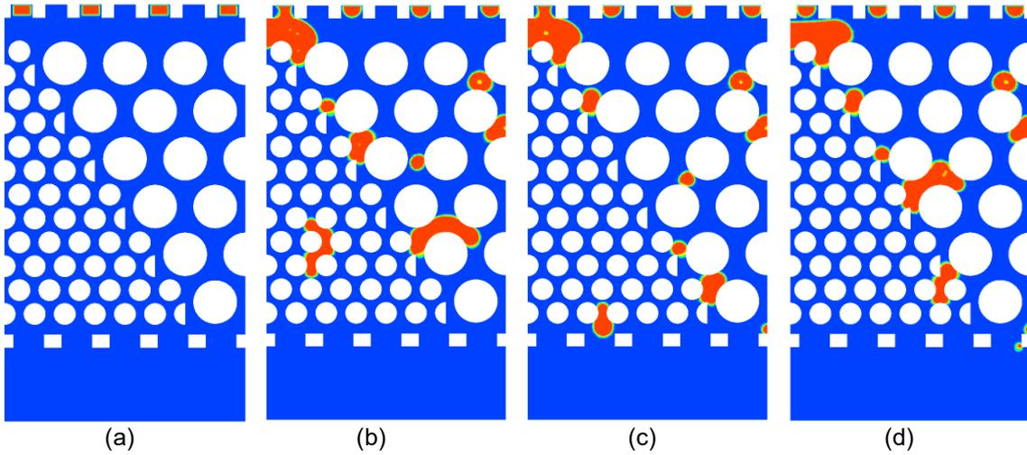
FIG 11 — Simulated slag flow in the packed bed with poor permeability region at different times: (a) 0 s, (b) 6 s, (c) 12 s, and (d) 18 s.
