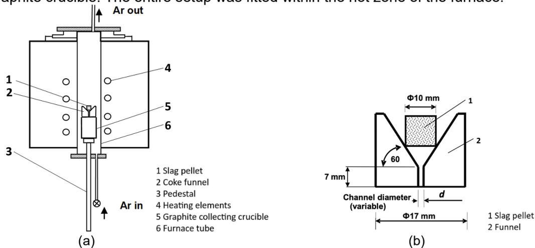
FIG 2 – Schematic diagrams of (a) the furnace arrangement for funnel analogue experiments and (b) a funnel and the placement of a slag pellet (George, 2013).
