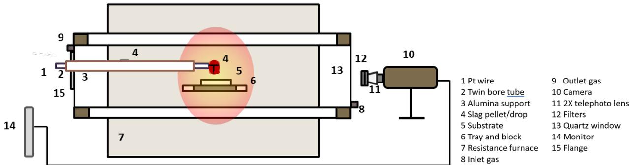
FIG 1 – A schematic of the sessile drop experimental set up (Abdeyazdan, 2016).
