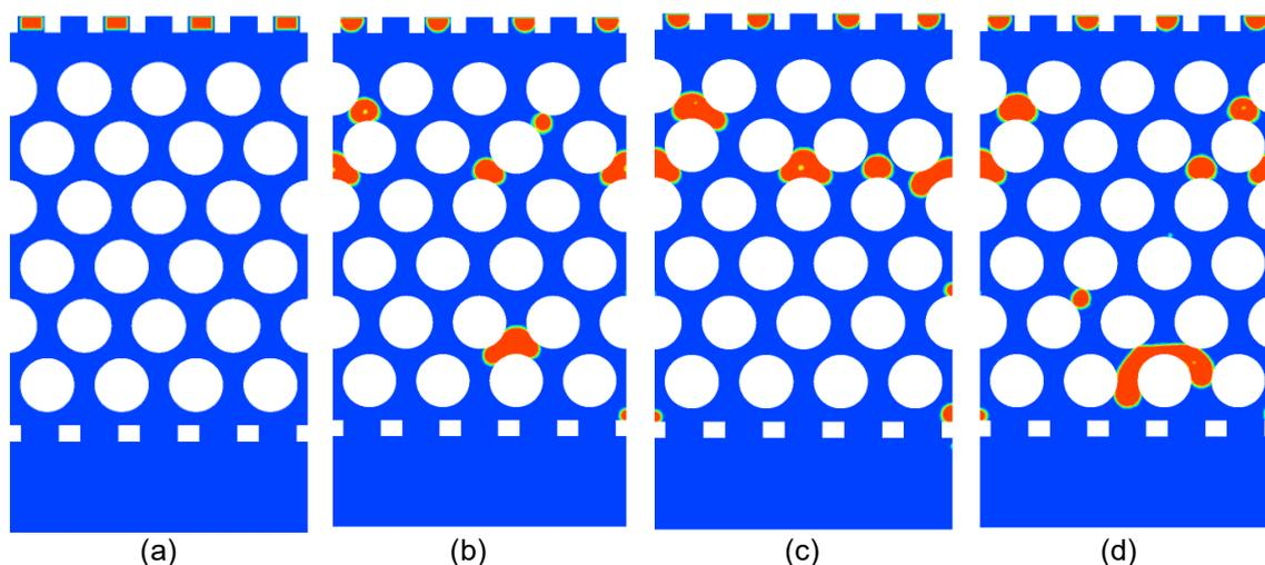
FIG 8 – Simulated slag flow in the base bed condition at different times: (a) 0 s, (b) 6 s, (c) 12 s, and (d) 18 s. Note that Slag 1 was used.
