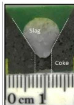
FIG 6 – Blocked slag droplet in coke funnels with a pore neck diameter of 4.5 mm.
