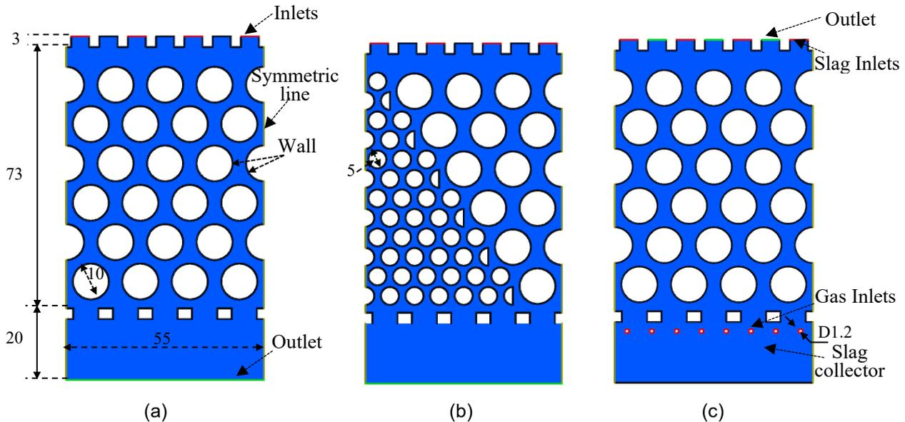
FIG 4 – 2-D computational domain for slag flow in the packed bed (a) base bed, (b) bed with deadman-shaped poor permeability region, and (c) counter-current gas and slag flow in the packed bed (unit: mm).
