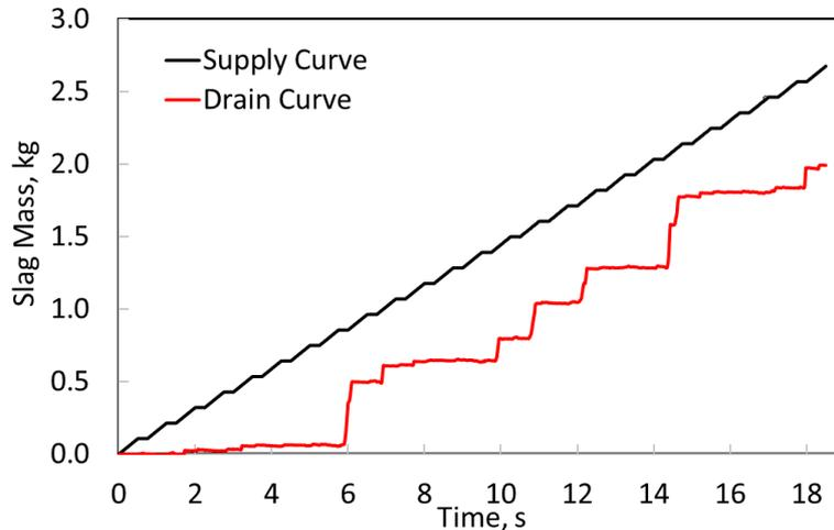
FIG 9 – A supply–drain curve from the simulation based on the base bed condition.
