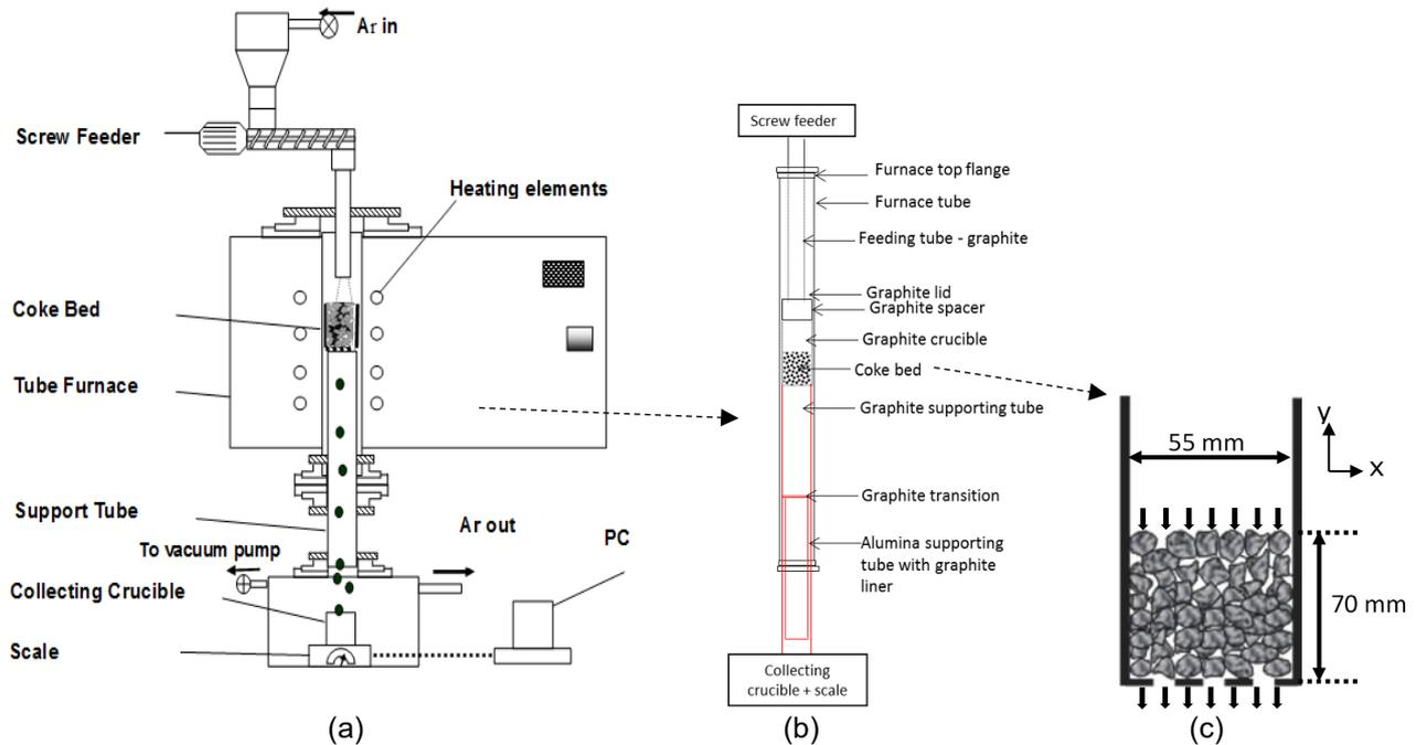
FIG 3 – (a) High temperature packed bed experimental facilities (George, 2013); (b) schematic of the detailed packed bed furnace arrangement; (c) a schematic of the coke bed.
