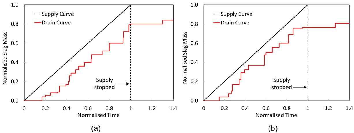
FIG 7 – Supply-drain curves of selected packed bed experiments of (a) Slag 1 and (b) Slag 2.
