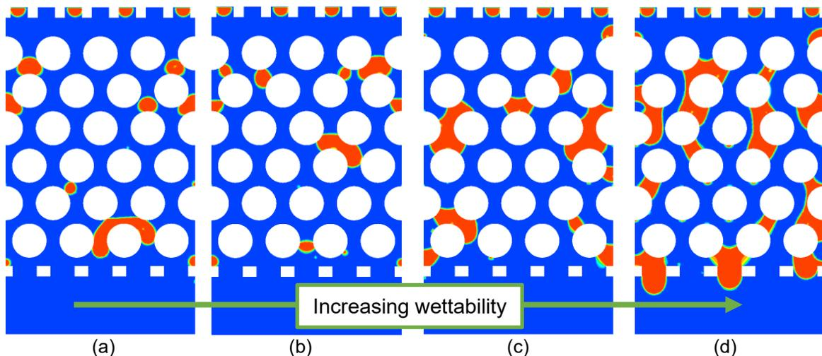
FIG 10 – Simulated slag flow in the packed bed at time  $t = 18$  s for different contact angles: (a) 157 deg, (b) 120 deg, (c) 90 deg, and (d) 60 deg.
