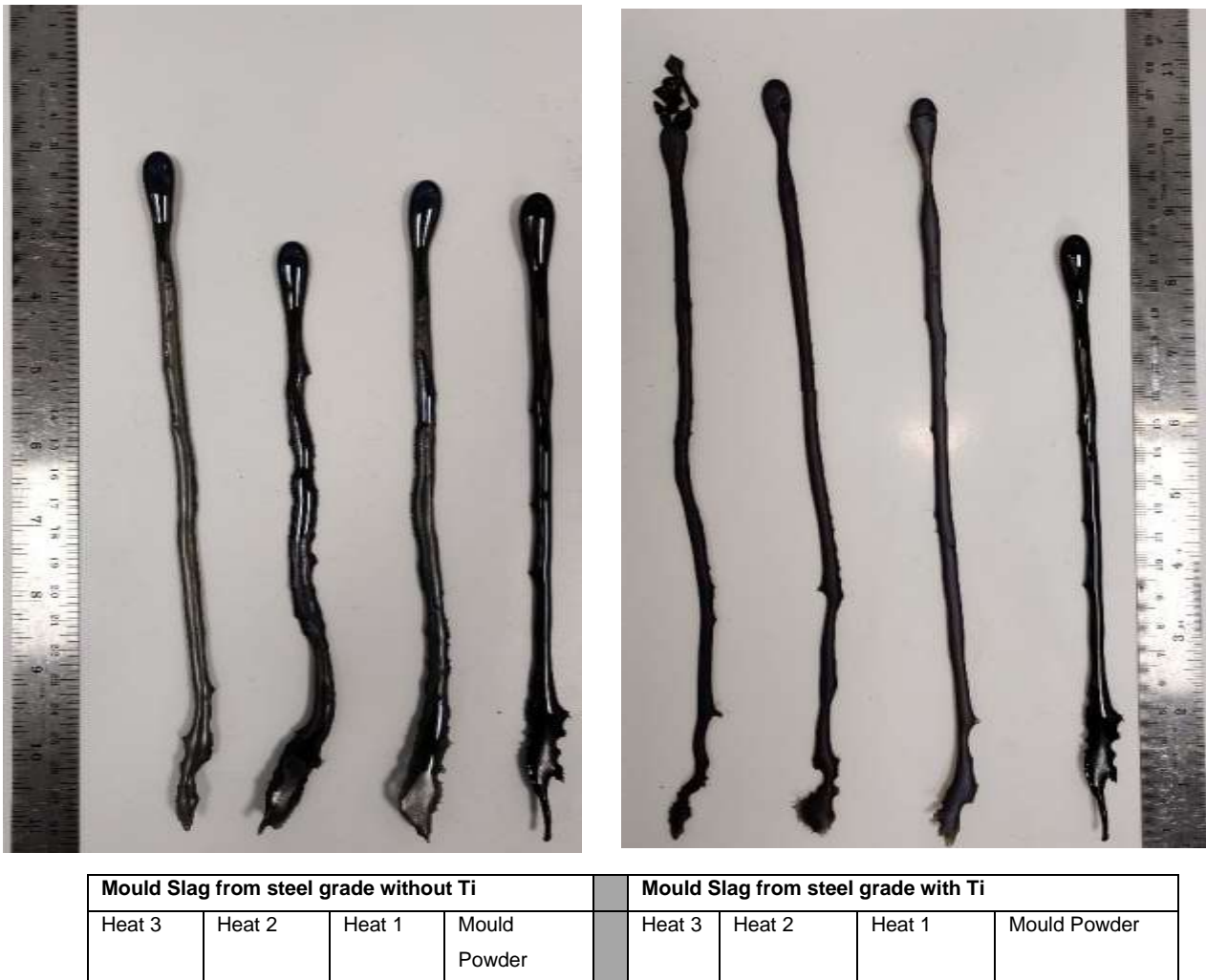
Figure 4: Fluidity of slag measured using inclined plane test method.
