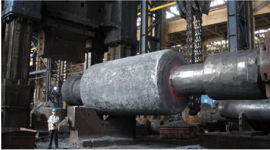
FIG 7 – Low-pressure rotor forging 408 t in weight maximal diameter 3650 mm forged from 715 tons conventional casted ingot of 30Cr2Ni4MoV (Courtesy of China First Heavy Industries)
