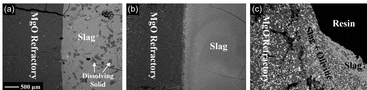
FIG 3 – Examples of secondary electron images from samples melted at 1500°C with an initial SiO<sub>2</sub>/MgO ratio in slag of 3.00 for melting times of: (a) 5 minutes; (b) 30 minutes; and (c) 120 minutes
