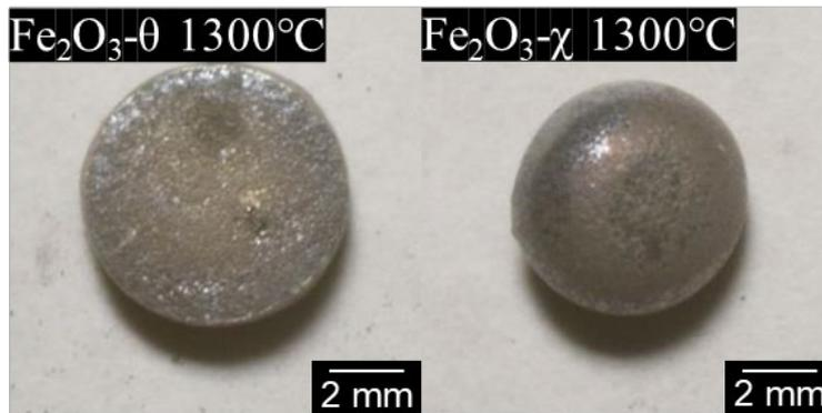
FIG 5 – Appearances of  $\text{Fe}_2\text{O}_3\text{-}\theta$  and  $\text{Fe}_2\text{O}_3\text{-}\chi$  after reduction heated up to  $1300^\circ\text{C}$ .
