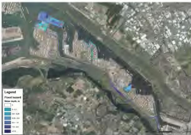
Figure 1 – Flood map climate scenario 2050 (+35cm SLR) for 1,000 years (left) and for 10,000 years (right) return period
