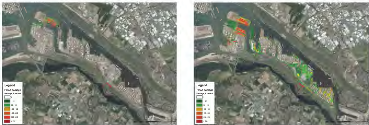
Figure 4 – Damage maps climate scenario 2050 (+35cm SLR) for 1,000 years (left) and 10,000 years (right) return period
