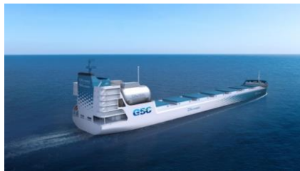
Ammonia-ready LNG-fueled bulk carrier (Planning and Design Center for Greener Ships website)
