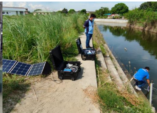
Testing of EWR box in a creek
