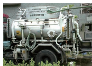
A vacuum truck with concentrating function
