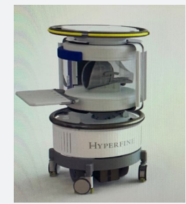
Swoop (Hyperfine, Inc)* - Portable ultra-low field MRI for brain imaging
