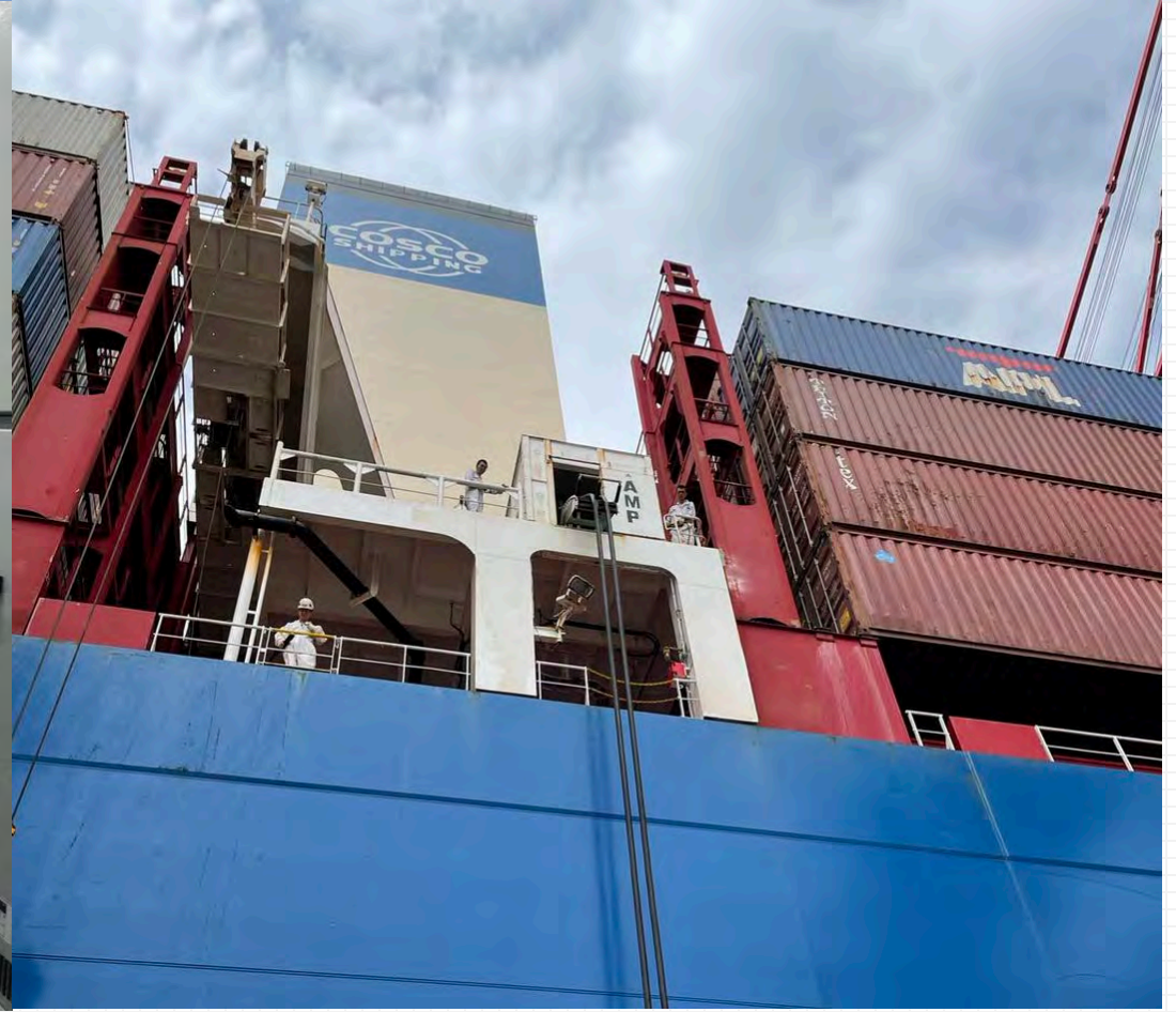
Shore-based power supply and ship connection operation
