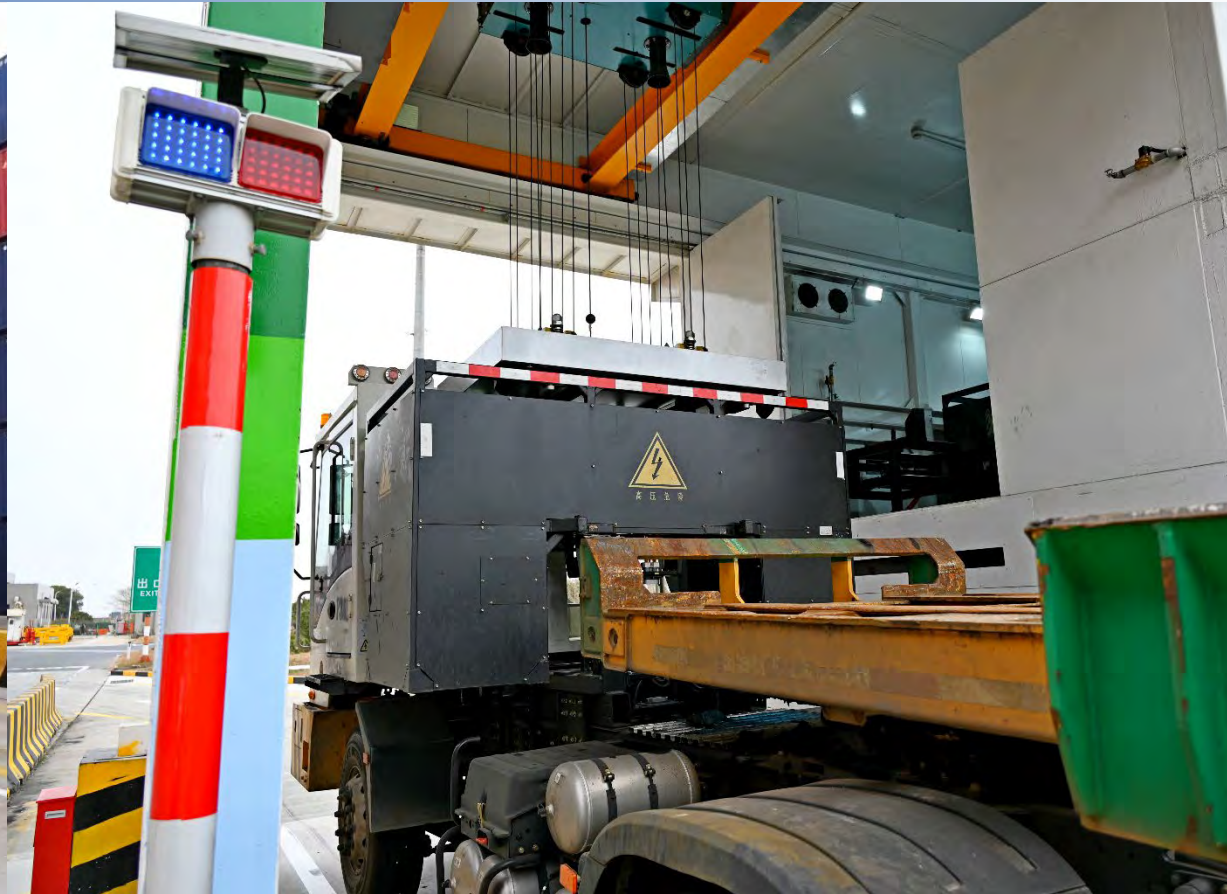
Power swapping operation for internal container truck
