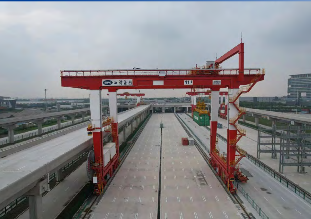
Yangshan Port Water, Highway and Railway Collecting and Dispatching Center (Double-layer operation process of full-automatic rail crane + automatic driving intelligent truck)
