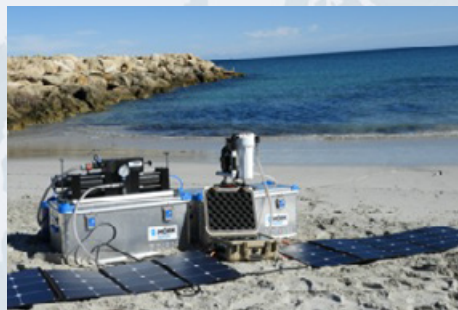
Portable unit 30 l/hr - treating sea and brackish water Perfect for rapid deployment as part of disaster relief
