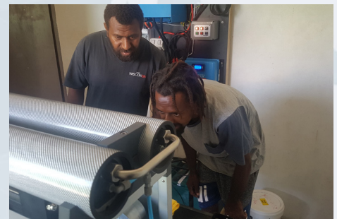
Community plant 250 L/hr - treating sea and brackish water Designed to provide clean water for health centres, schools and communities
