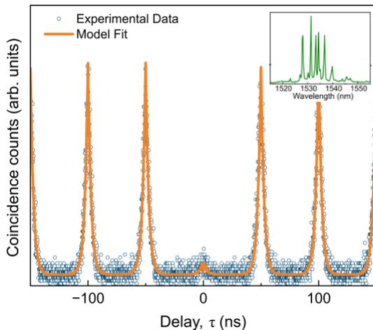
Fig. 2. Second-order auto-correlation measurement,  $g^{(2)}(\tau)$ , of the peak at  $\lambda = 1531$  nm (see inset) from a single nanowire quantum dot device. The fit (orange curve) is generated using a stochastic model used to describe the photon emission statistics [3].
