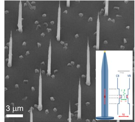
Fig. 1. Scanning electron microscopy image of an array of nanowire quantum dot C-band single photon sources. Inset shows a schematic of the  $\text{InAs}_x\text{P}_{1-x}$  dot (dark red) in a  $\text{InAs}_y\text{P}_{1-y}$  rod (light red) device along with the associated band structure.
