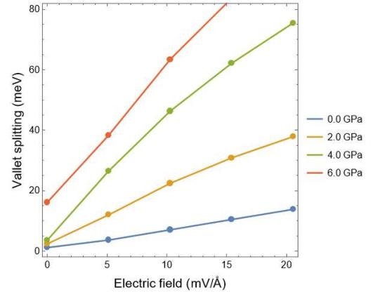
Fig.1. Valley splitting as a function of electric field with various strengths of stress.
