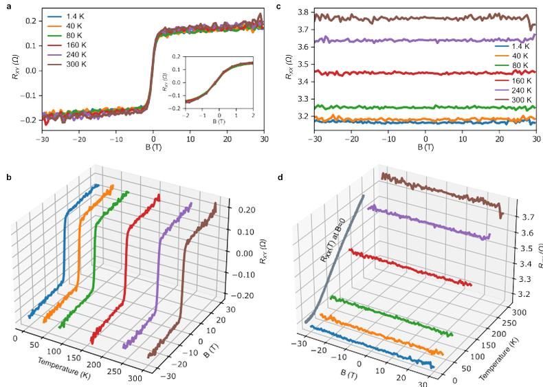
Fig. 1. **Temperature and magnetic field dependences of the Hall and longitudinal resistances for a 68 nm device.** a, Hall and c, longitudinal resistances as a function of the magnetic field at various temperatures ranging from 1.4 K to 300 K. The inset in a is the zoom-in for the data between  $\pm 2$  T. b, d, 3D plots of the same curves in a and c respectively.
