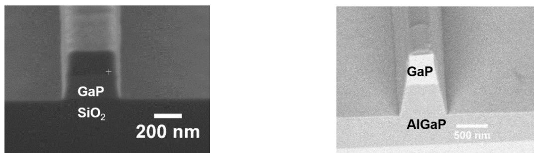
Fig.1. SEM image from a) a nanowaveguide of GaP on insulator. b) a nanowaveguide of GaP/AlGaP/GaP.
