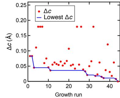
Fig. 2. Actual  $\Delta c$  values and the lowest experimental  $\Delta c$  plotted as a function of growth run.
