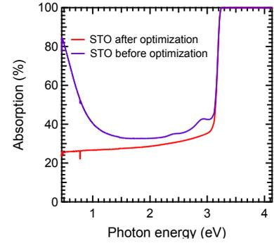
Fig. 1. Optical absorptions of STO films before and after BO.
