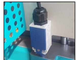
Hood Safety Switches
