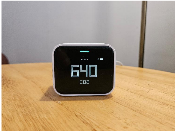
Qingping Lite: PM, CO 2 , T, RH
