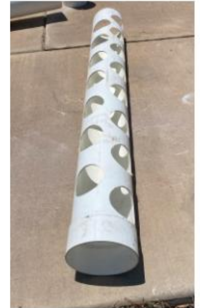
DN50 irrigation pipe with media support at 300mm
