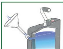
Use a watering can and funnel to fill the steam generator with clean tap water.
