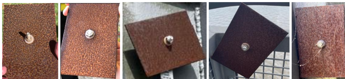
Fig. 7 – UWS plates in different environments after 13-18 months.
